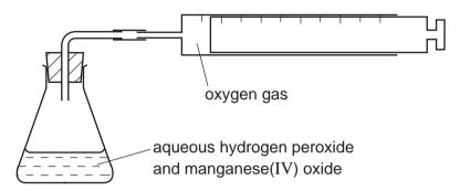
$40\,\mathrm{cm^3}$  of aqueous hydrogen peroxide was put in the flask and 0.1 g of small lumps of manganese(IV) oxide was added. The volume of oxygen collected was measured every 30 seconds. The results were plotted to give the graph shown below.
